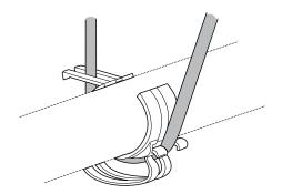
Non-slip abrasion protection between truss and suspension element.
