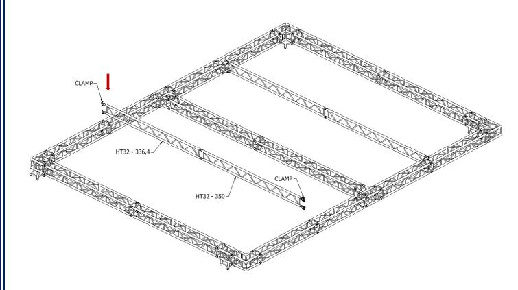
The exact position of the HT32-336,4 will be defined in the next step using inclined tubes.
